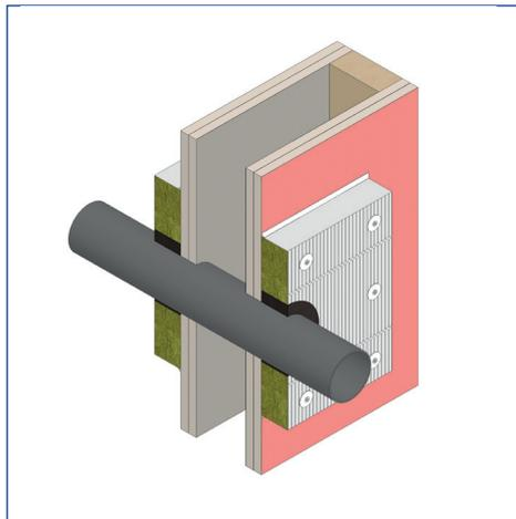
FB750 double batt patten fit + FS709 HP seal: E1120
